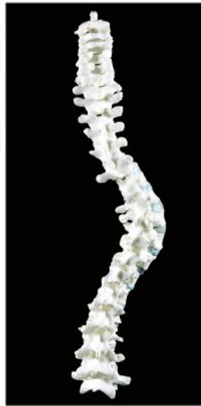
3D model of spine with replica polymer vertebrae created by laser sintering
